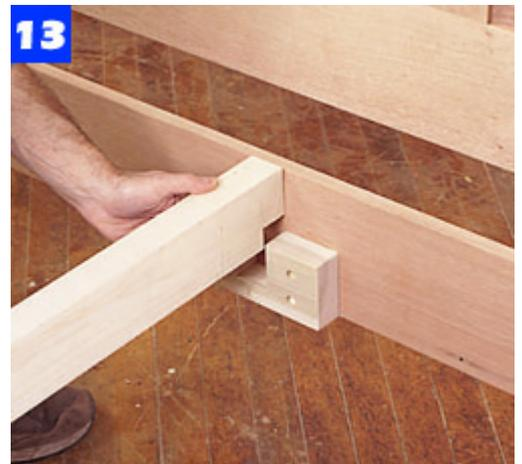
After engaging the side rails with the head- and footboards, slide the slat-support beam into position.
