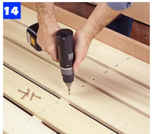
Check that the bed frame is square before installing the slats. Then, secure each slat with 1-1/2-in. No. 8 screws.
